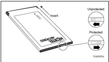
3 Adjust the read-write protect switch.
